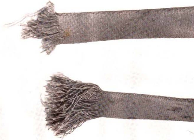
Figure 18 Strap Failure Caused by Rubbing Against Metal
