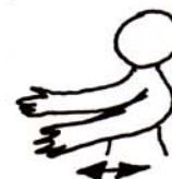
MOVE LEFT Extend right arm horizontally side- ways. Swing left arm in front of body to indicate direction of move- ment; repeat
