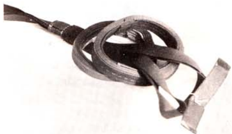
Figure 9a. 1st Step-Choker hitch
